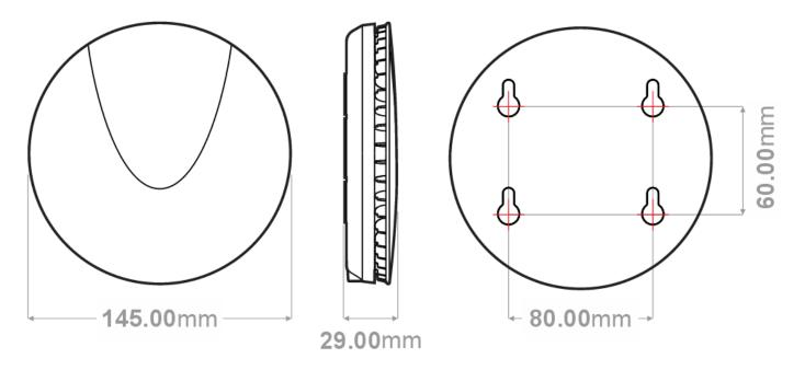
Dimensions above are shown with the cover in the closed position. Dispenser depth in the open position: 34 mm.
